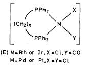
various bonds are eclipsed,<sup>8</sup> slightly increasing strain in these systems. This is reflected in the bond lengths (Pd-P).<sup>8</sup> The <sup>31</sup>P n.m.r. chemical shifts and coupling constants  $[{}^{1}J(Pt-P)]$  for these complexes, as well as for complexes of Pt<sup>II</sup> with (1)—(3),<sup>9</sup> also vary greatly.
